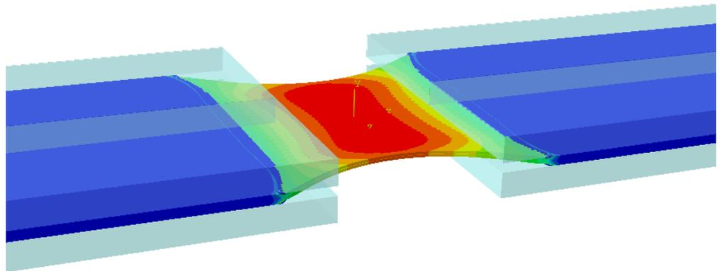
**Fig. 4:** Simulation of debonding with cohesive zone elements for a PVB-laminated glass in through-cracked tensile test
