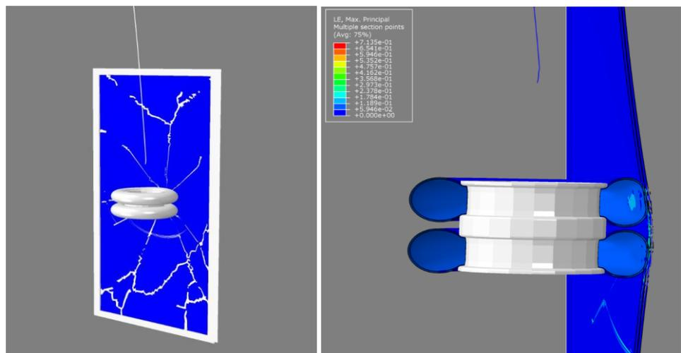
**Fig. 5:** Detailed simulation of double tire pendulum impact on laminated glass
