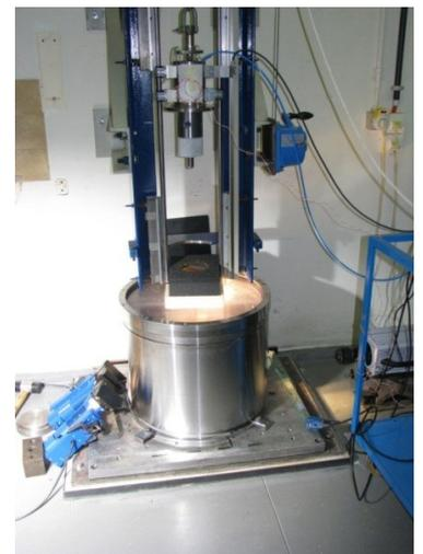
**Fig. 1:** Small- scale drop weight. Force sensor, accelerometer and magnetic strips for displacement measurement on impactor; strain gauges and high speed imaging (up to 250000 fps, from sides and bottom) can be applied to test piece.
