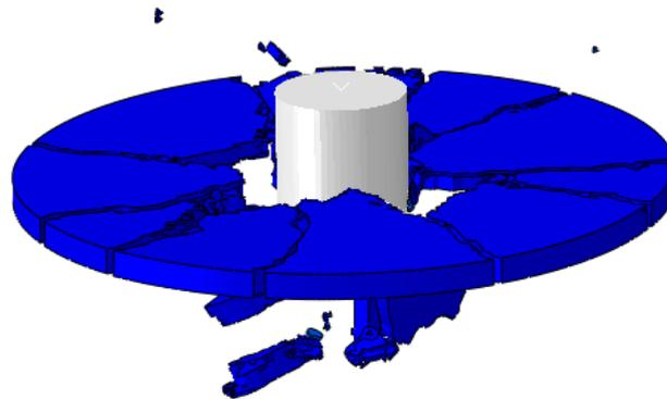
**Fig. 3:** Dynamic cracking simulation of small monolithic glass plate in impact by drop weight
