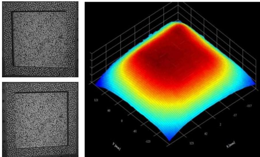
**Fig. 2:** Digital Image Correlation of glass panel under 20g C4 explosive blast load: high-speed camera images from 2 angles (left), 3D deformation of processed data (right)
