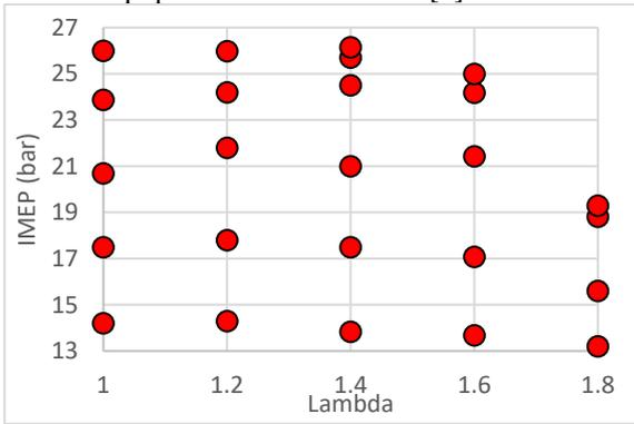
Figure 1. 25 operating points of the test.
