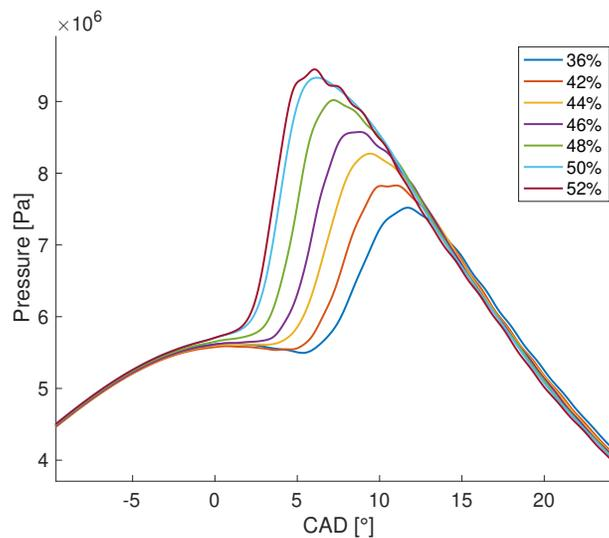
**Figure 1:** Pressure curve shift in the range 36% - 52% oxygen content
