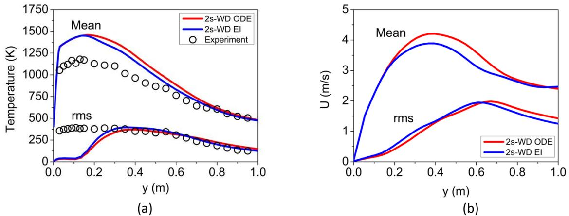
Figure 2. Mean and rms centerline (a) temperature and (b) axial velocity for UMD test case with different chemistry solvers.
