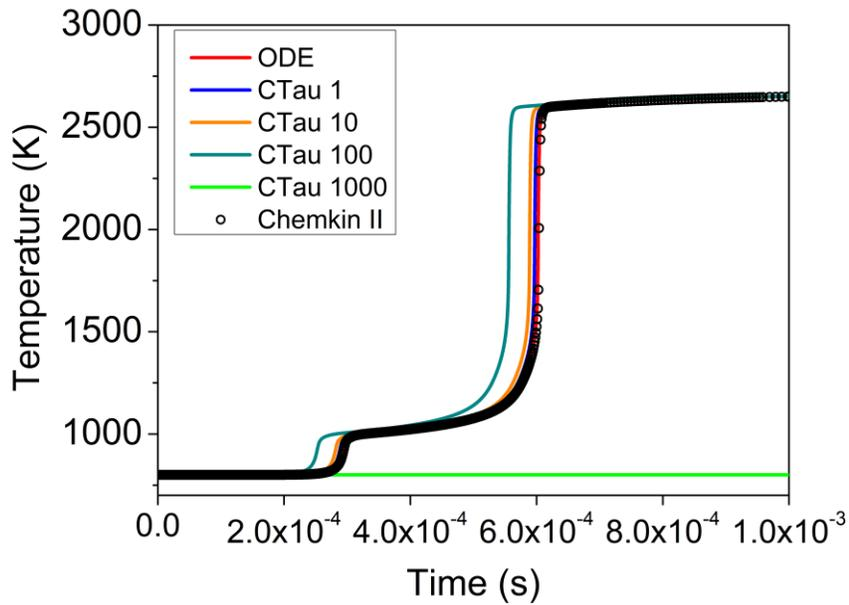
Figure 1. Simulation result of the benchmark test case (*n*-heptane); temperature profile across different chemistry solvers
