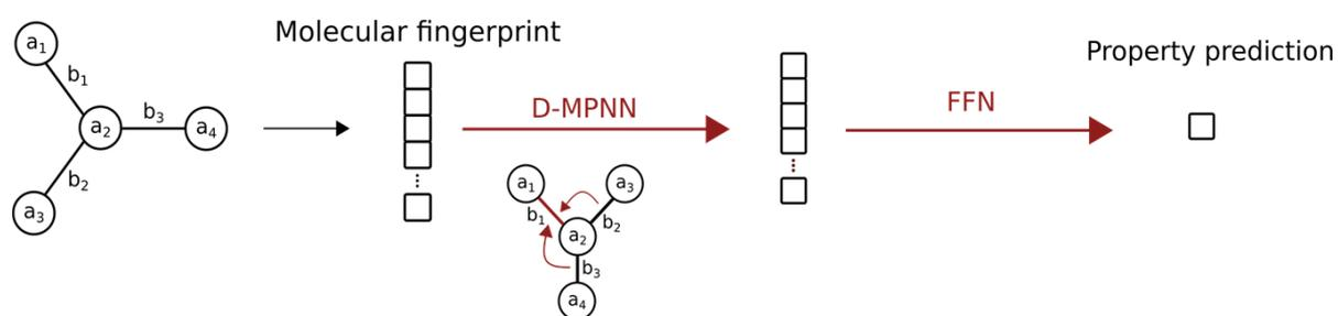
Figure 2. Machine learning model architecture of a message passing neural network
