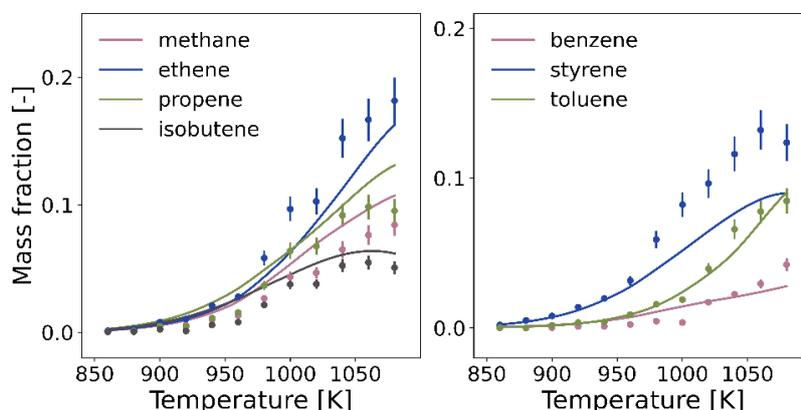
Figure 1. Mass fraction of the main product species from the pyrolysis of a Jet-A surrogate, comparing experimental measurements (symbols) and model simulations (lines).
