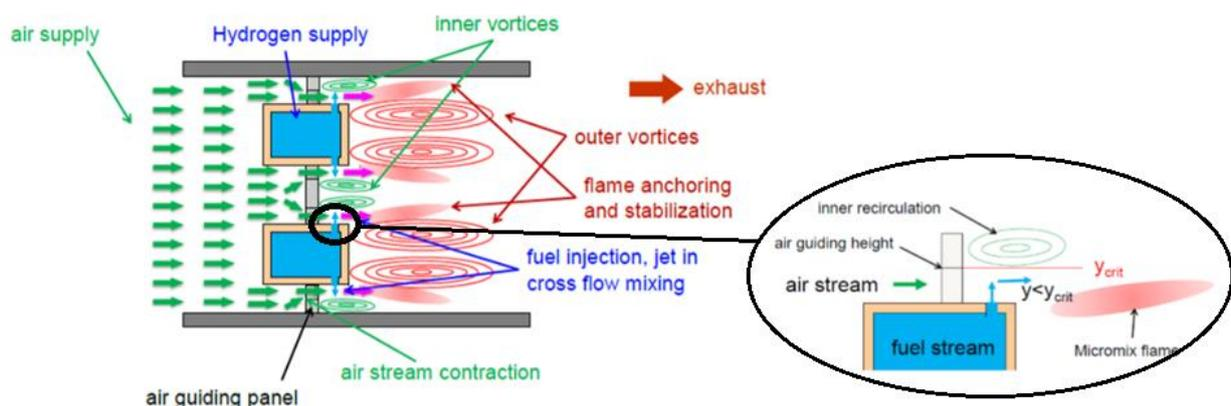
Figure 1: Micromix nozzle schematic overview [2]
