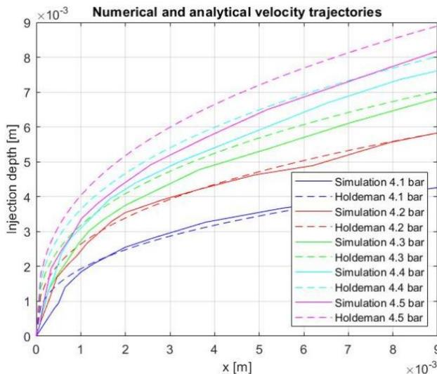
**Figure 3:** Numerical and analytical velocity trajectories at different hydrogen inlet pressures
