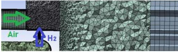
**Figure 2:** Mesh of the single nozzle micromix combustor test geometry
