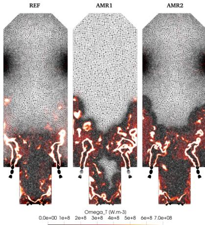
Figure 2: Comparison of the instantaneous reaction rate fields, superposed to the mesh, in a 2D cross section plan along the axial axis, highlight that in the REF case (left) the flame extends beyond the pre-defined refined zone, while in both AMR1 (center) and AMR2 (right), the mesh is refined around the flame.
