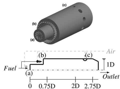
Figure 1: 3D and 2D representations of the simplified geometry of the Turbec T100 mGT combustor where the total combustion air flow rate is distributed as follows: 4% in the 12 pilot injectors for air (and 6 for fuel) for the diffusion pilot flame (a), 21% in the 30 main premixed injectors (b) and 75% through the 9 dilution holes (c).
