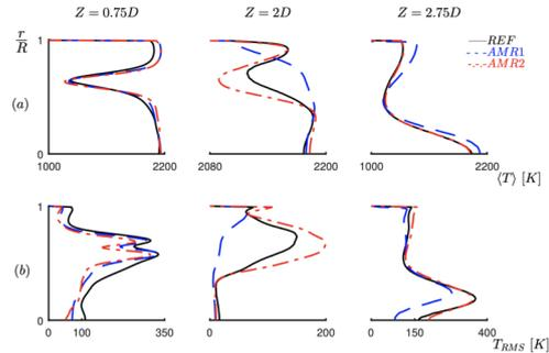
Figure 3: Comparison of azimuthal time average and RMS temperature (a and b) between the reference (in black), AMR1 (in blue), and AMR2 (in red) cases in 3 positions taken along the combustion chamber:  $Z=0.75D$ ,  $Z=2D$ , and  $Z=2.75D$ , demonstrating the benefits of applying AMR in the flame region.
